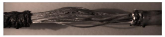
Unprotected cable 60 second propane/air torch burn All conductors burned and shorted
