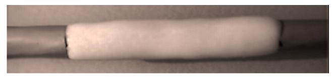
Coated with 0.030" CylaTherm N-30/RTV Silicone (50/50)
