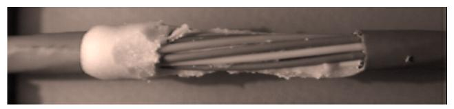
Cutaway of burned coated cable
